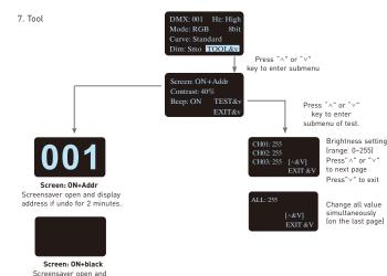
Fast self-testing function: press "^"or "\" keys simultaneously for 2-3 seconds under any page, decoder will enter self-testing function.
