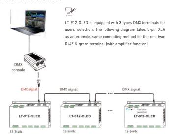
If the recoil effect occurs because of longer signal line or bad line quality, please try to connect 0.25W 90-120Ω terminal resistor at the end of each line.
